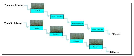
Fig. 1 Schematic layout of Nimr's train A & B reed beds
