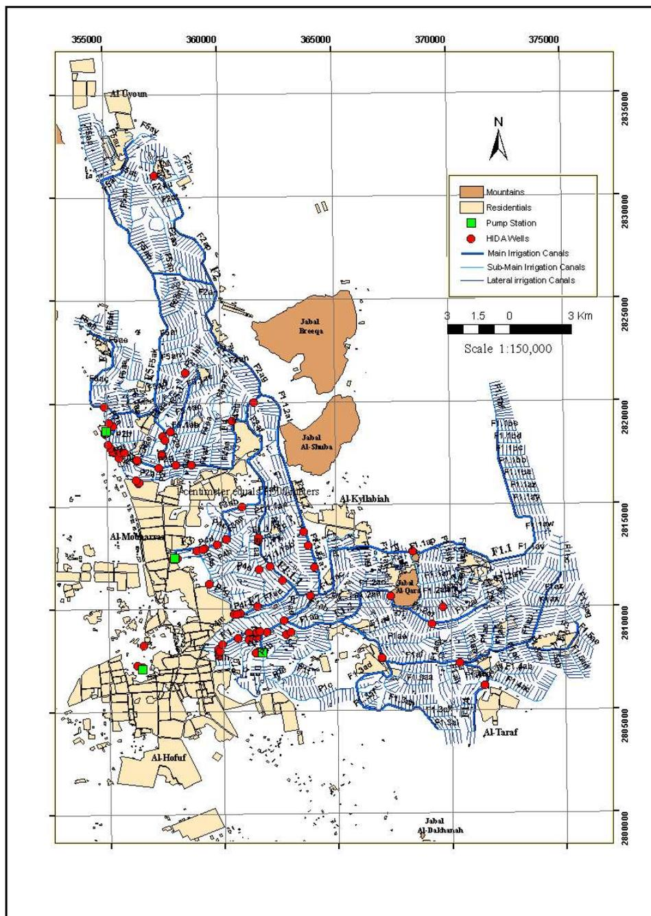
Fig. (3) Irrigation system and water wells in Al-Hassa Oasis
