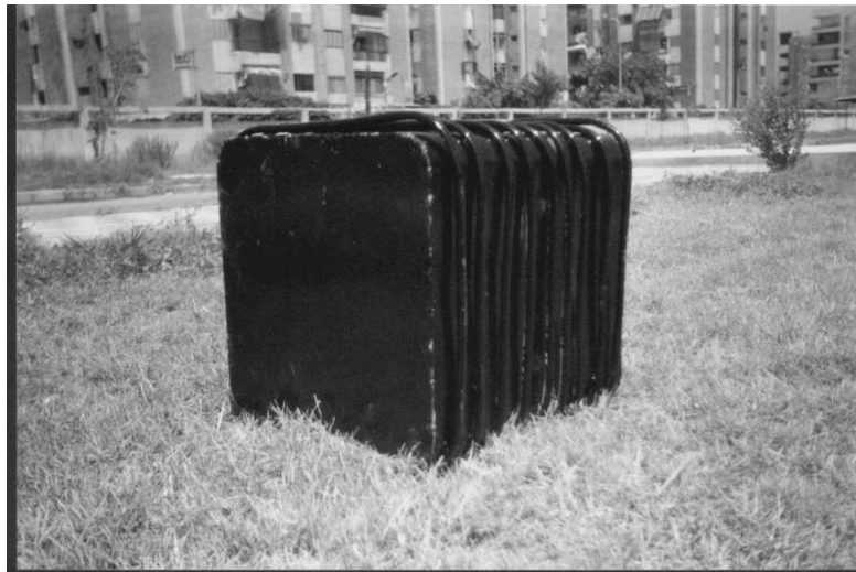
Fig.7 Central receiver with single tube copper coil on the absorber surface
