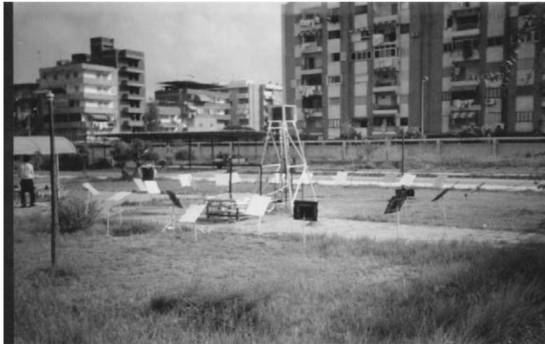
Fig.2 Photo of the test rig with 28 heliostat (arrangement 1)
