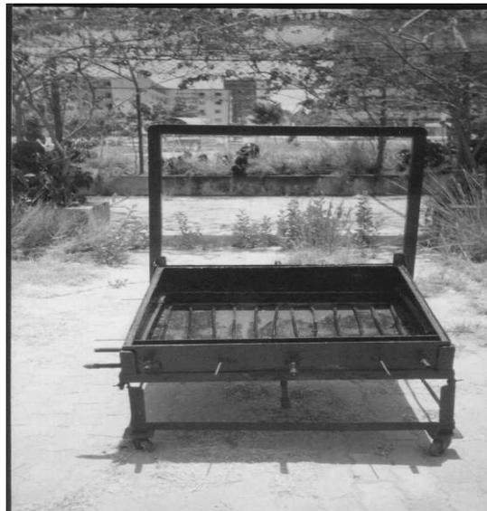
Fig.5 Solar still with single tube copper coil on the bottom
