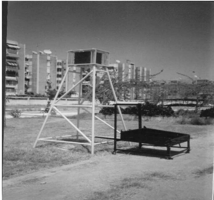
Fig.6 The central receiver with the steel construction tower
