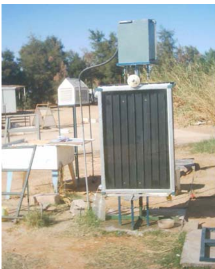
Figure 1 indirect solar still
