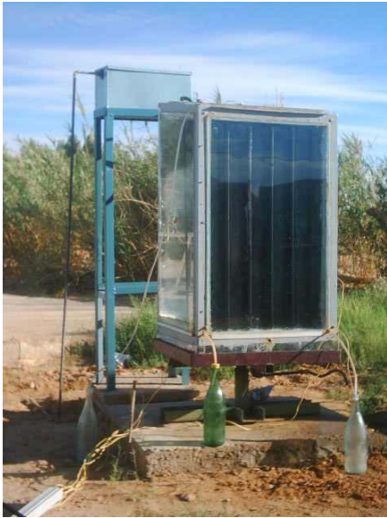
Figure 10 Direct and indirect vertical solar still under test
