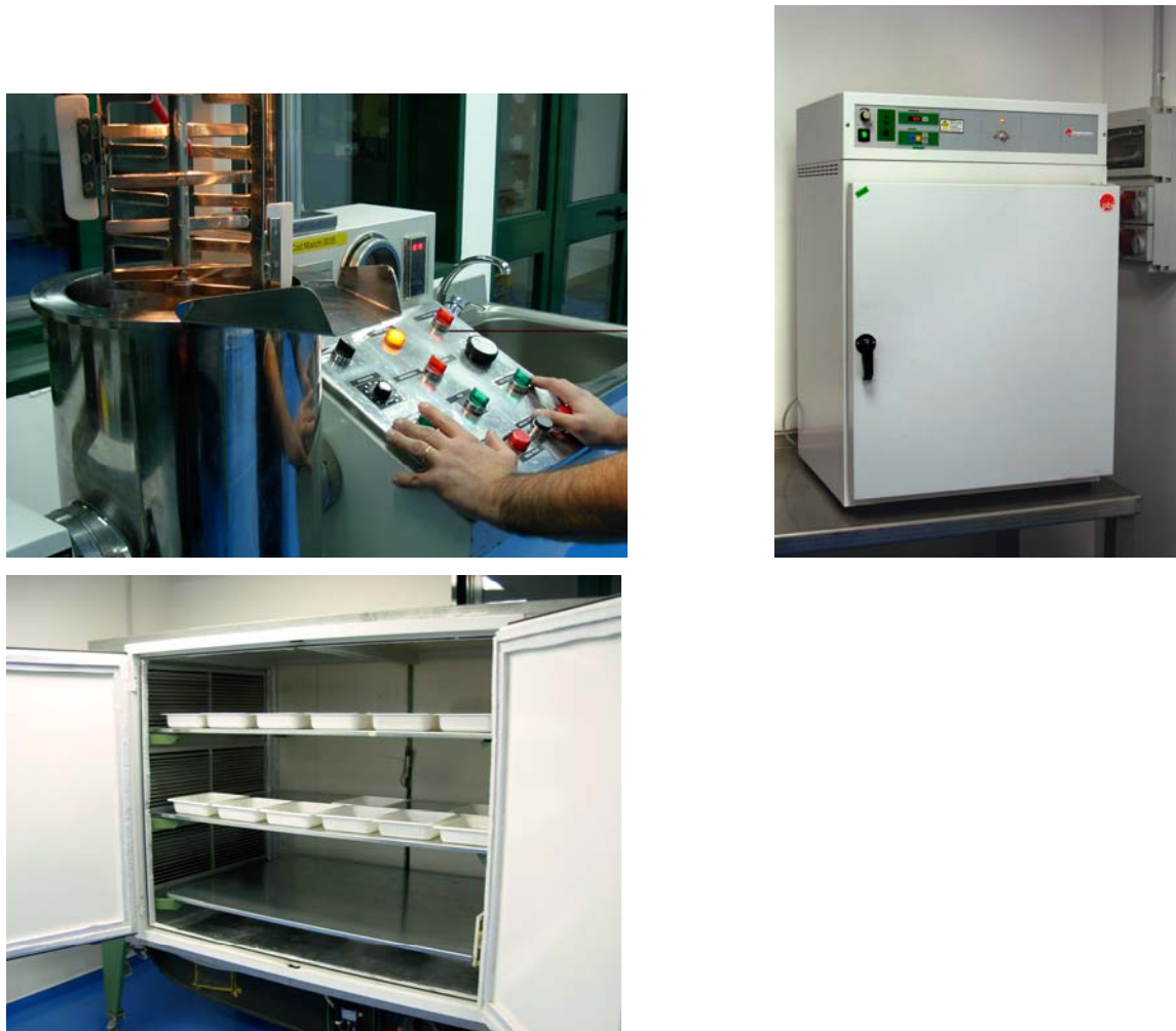
Figure 12. The mixing stage (up, left); the crosslinking stage (up, right); the desiccation stage (down).
