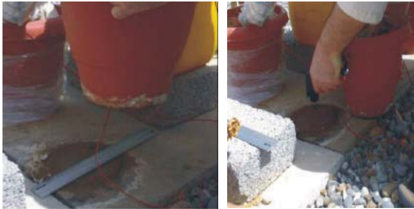
Fig. 6: The measurement of the roof surface temperature by a thermocouple and radar under the pot
