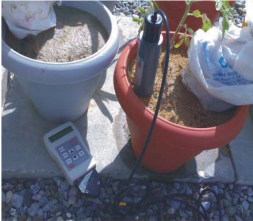
Fig. 4: Moisture content reading by \theta -probe device
