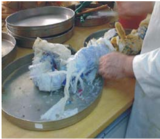
Fig. 8: Visual inspection and sensation of the opened siphon (the external layer of plastic exposed to direct solar radiation dilapidated)
