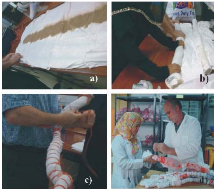
Fig. 2: Preparation of siphons: cotton tissue with soil core a), rolling b), wrapping c), plastic covering d)
