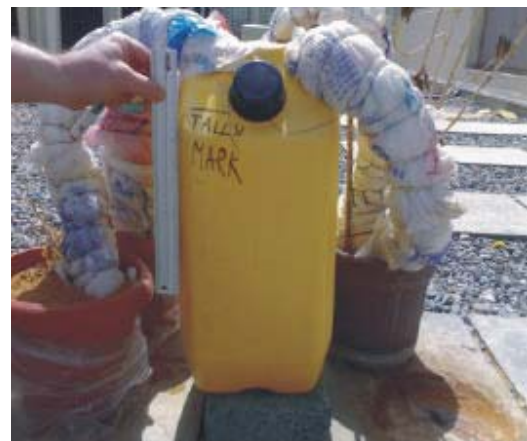
Fig. 3: Container with a "tally mark" up to which water was regularly added
