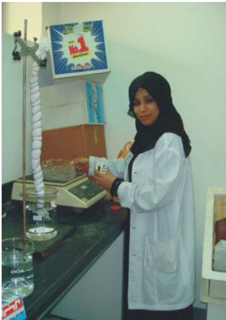
Fig. 5: Measurements of accumulating mass of water imbibing into an initially dry vertical siphon
