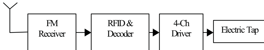
Fig. 2: Block diagram of the field station of the implemented system
