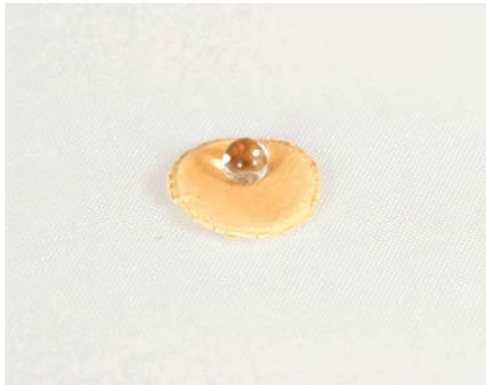
Fig. 2: Picture of the water droplet on the membrane surface grafted with the fluoroalkylsilane.
