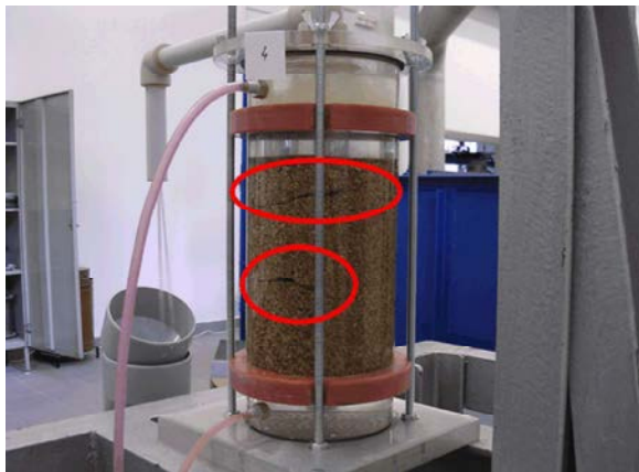
Fig. 7: The disruption of the specimen starts with single “cracks” (heave) due to the uplift force - experiment 1.
