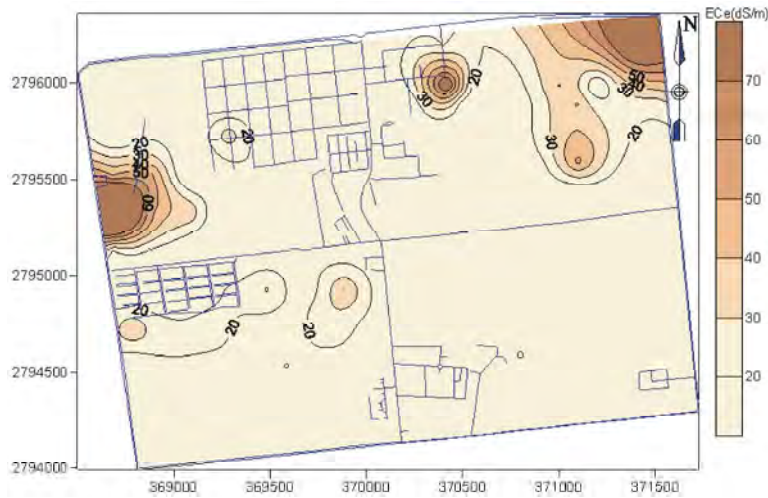
Fig. 4b: Spatial distribution of measured electrical conductivity for the collected soil samples at interval of 30-40 cm Al Hassa area, KSA
