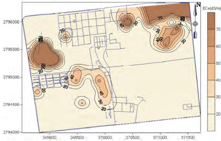
Fig. 4a: Spatial distribution of measured electrical conductivity for the collected soil samples at interval of 10-20 cm, Al Hassa area, KSA
