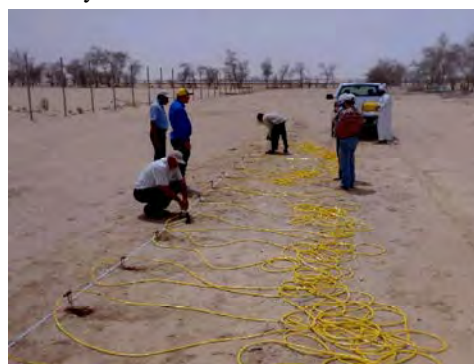
Fig. 2b: The SuperSting R8/IP 8 resistivity system and the electrode arrays, during the mapping of the hardpan layer at the study area.
