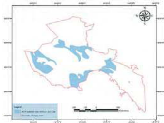
Fig. 8: AGR suitable sites without land use/land cover layer obtained by using AND Boolean operator
