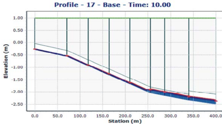
Fig. 2: Longitudinal profile in the sewer pipeline from segment CO-19 to segment CO-10 at time 10 AM.
