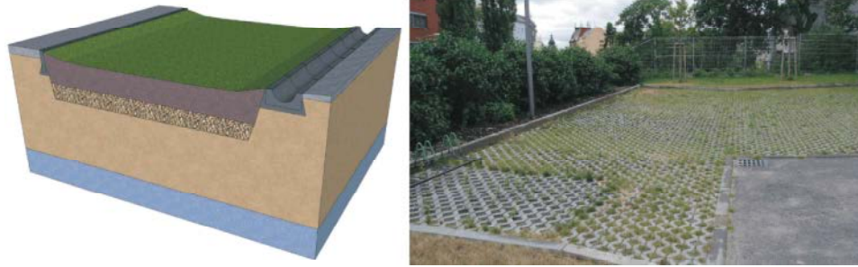
Fig. 1: Surface infiltration –left scheme [14], right Brno University of Technology, CR
