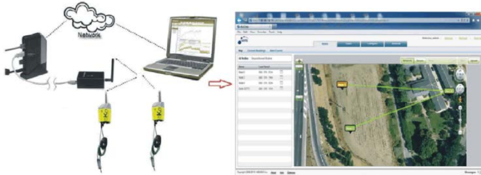
Fig. 3: Scheme for the wireless sensors network components and the nodes deployment in the experimental site
