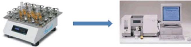
Fig. 2: Batch adsorption process and measurement of Cr (VI) ions by AAS
