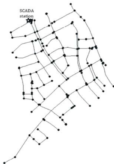
Fig. 2: Water distribution network of the PSA for EPANET model application
